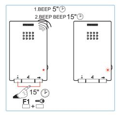
2. Press the F1 button and the wo button simultaneously for 15 seconds until you hear a double tone (BEEP BEEP) and release. After 5" you hear a BEEP and after 10" you hear a BEEP BEEP.
