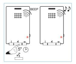
1. The user should start in the "Ringtone Selection" configuration menu. from the outdoor panel". Press and hold the button for 5 seconds until you hear a "beep" then release, a ringtone will sound on the current panel. While in this mode:
