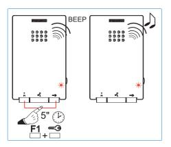
Press the F1 and the button simultaneously for 5 seconds until you hear a tone (BEEP). Release.
