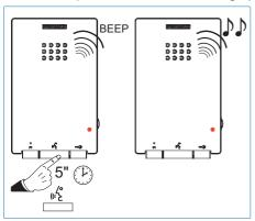
1. The user should start from the "Ringtone Selection" configuration menu. Press and hold the d button for 5 seconds until you hear a "beep" then release, a ringtone will sound on the current panel. While in this mode:
