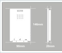
Telephone Dimensions (Height x Width x Depth\*.): 146 x 90 x 20 mm
