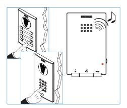
3. Press the button/residential call code from the panel. A confirmation tone will sound on the telephone. The telephone is programmed, (red led off)
