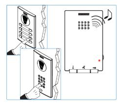
Press the button/residential call code from the panel. A confirmation tone will sound on the telephone. The telephone is programmed, (red led off)
