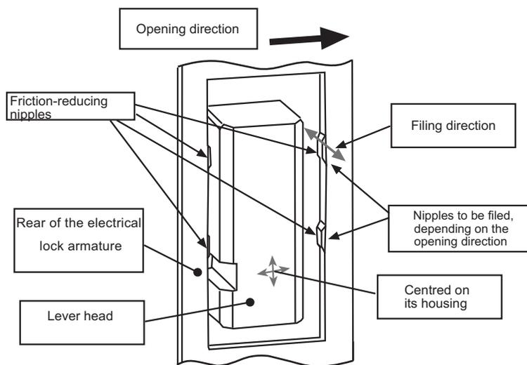
The distance between the two faces has to be as great as possible (**between 3 and 4 mm**) so that the pressure applied by the door handle on the brass window is controlled. This also increases the lifetime of the product and allows for smoother closing.
