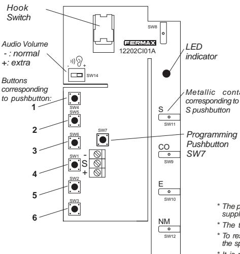
**1. Open the telephone cover, keep pressed the hook switch and press the programming pushbutton once (SW7).**
