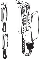
This call can be attended from any telephone. Just hung up the telephone and press the button **E**.
