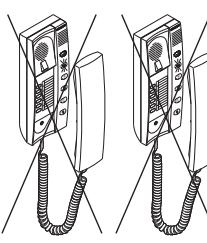
During the conversation the door release can be activated pressing the button **H**)
