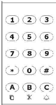
1. Key in the number of the block or sector where the Guard Unit is installed. Not necessary if it belongs to the same block.
