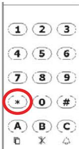
You can know the name or number of the person or flat that has made the call simply by pressing the '\*' key of the Guard Unit keypad. This will only be valid if this telephone is assigned to the users list. This information will be shown for 2 seconds.
