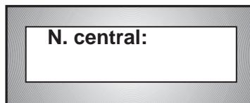
2. Key in the number of the block where the Guard Unit the calls are to be transferred to, using 2 digits at all times.
