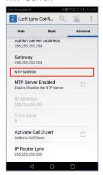
**NTP SERVER**. Allows the NTP server to be used or not for the automatic update of the date and time.
