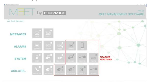
This main screen shows a series of icons, grouped into 4 sections (MESSAGES, ALARMS, SYSTEM and MANAGEMENT), which allow the user to access the corresponding function, as explained in the following sections of this manual.
