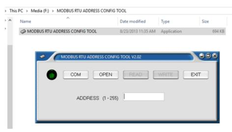
Click the "COM" button, select the "SERIAL PORT" number of the RS485 adapter. Port settings to be selected as shown in the figure below.
