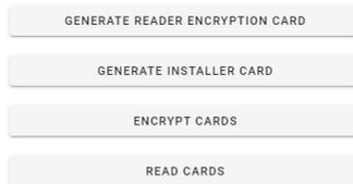
Finally, present the DESFIRE FERMAX proximity card you wish to encrypt to the DESFIRE desktop reader. This card will be encrypted as an INSTALLER card with the codes of the distributor and installer.
