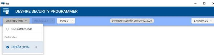
After adding the distributor certificate, the *DESFIRE SECURITY PROGRAMMER* PC software will allow you to encrypt a card to use for DESFIRE reader encryption.
