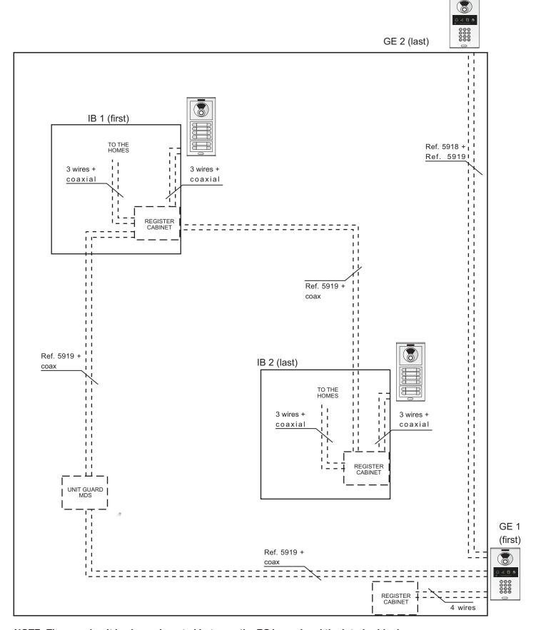
NOTE: The guard unit is always inserted between the EG1 panel and the interior blocks.
