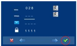
Select the programming option from the monitor VDS (2). The selected option is displayed with the white line under the icon.
