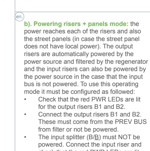
**b). Powering risers + panels mode:** the power reaches each of the risers and also the street panels (in case the street panel does not have local power). The output risers are automatically powered by the power source and filtered by the regenerator and the input risers can also be powered by the power source in the case that the input bus is not powered. To use this operating mode it must be configured as followed:
