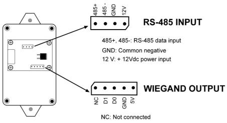
D0, D1: 26 Bit / Burst data output
